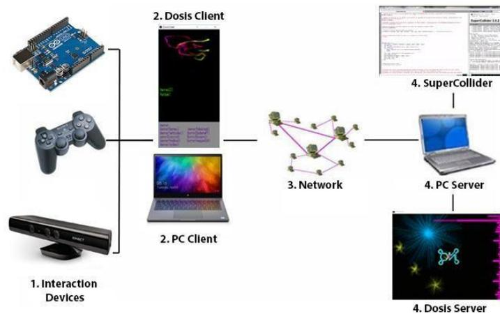
Figure 2. Client – Server connection scheme.
