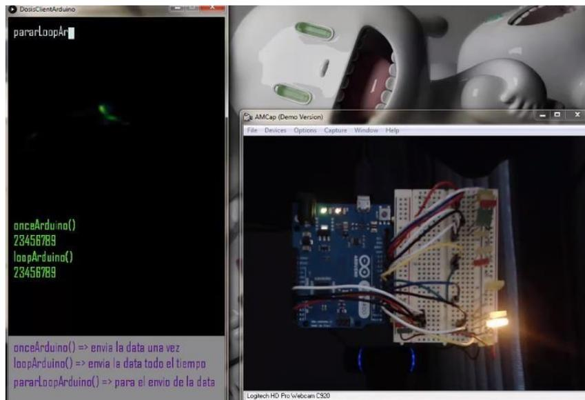
**Figure 5.** The letter typing on Dosis, turns on the led in Arduino. (<https://vimeo.com/282589746>)
